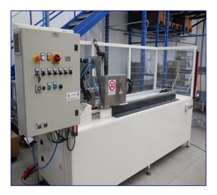
This is an automatic machine that binds the flaps packet. It automatically compresses three to six packs of flaps through a hydraulic cylinder, after which they are cut, glued with Hot Melt and finally cooled with X Air system.
