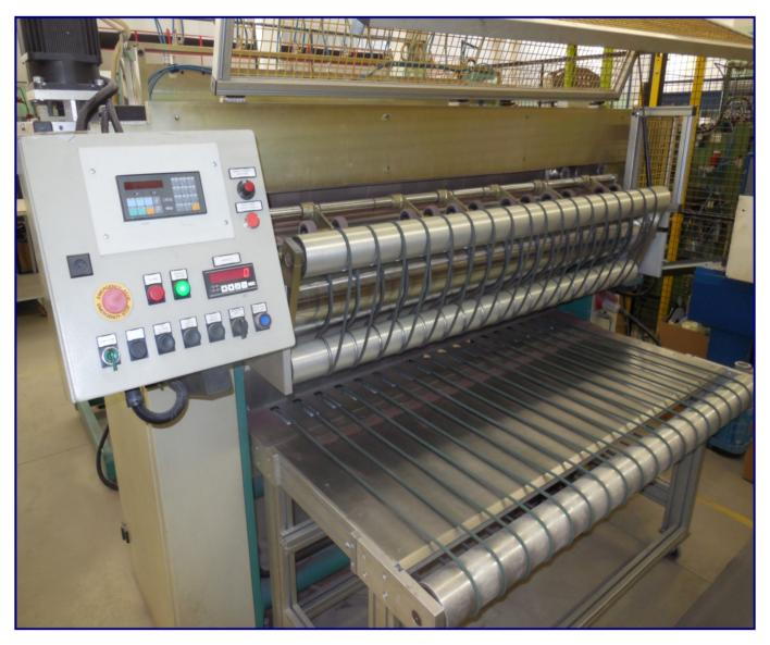
This automatic machine cuts flaps made of non-woven fabric, paper or cloth with the same height as the original roll; the maximum working width is 2000 mm. This system cuts a pre-set number of flaps that are used to assemble a roller in full automatic mode. The cutting is performed by means of a circular blade that, when shifted by a servomotor, performs the cut with great precision and speed. Flaps are then piled up in a buffer container and ready to be collected and processed.
