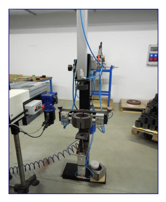
This concentric compression machine is designed for the insertion of the non-woven wheel manufactured by SMA-TFN and SMA-TFNW machines into a metal mold. Through simultaneous closing of two pneumatic jaws, the machine homogeneously compresses the material and inserts it into a retaining cylinder.
