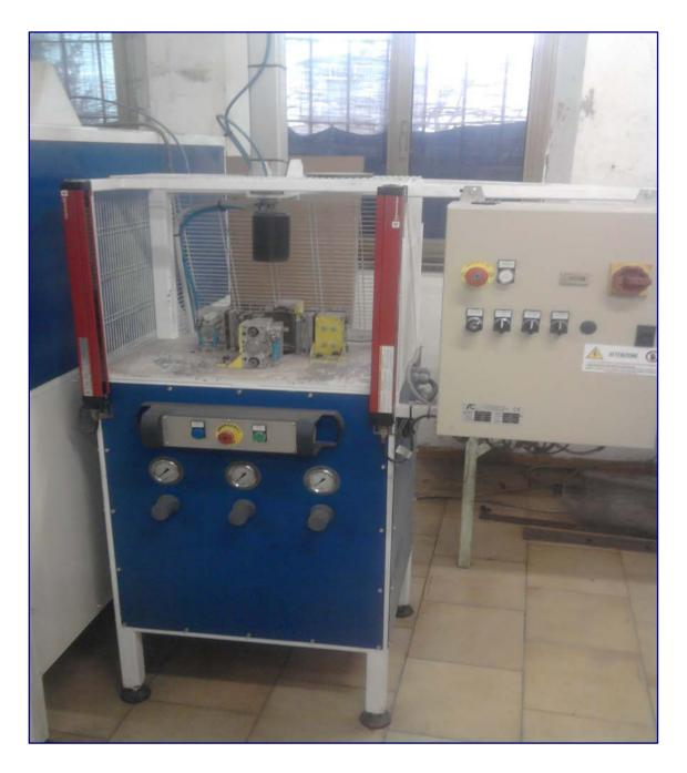
This concentric compression machine is designed for the insertion of the non-woven wheel manufactured by SMA-TFN and SMA-TFNW machines into a metal mold. Through simultaneous closing of four pneumatic jaws, the machine homogeneously compresses the material and inserts it into a retaining cylinder.
