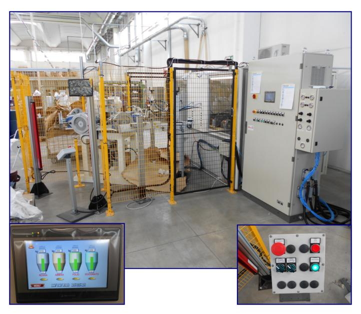
This machine is designed for the automatic bonding of flap wheels with flange. Its versatility allows to manufacture wheels whose diameters go from 110 mm to 350 mm.
