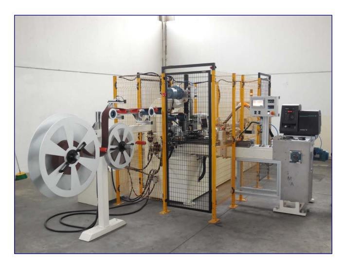
This is a new generation automatic machine for the production of wheels in non-woven fabric and combined non-woven + cloth.
