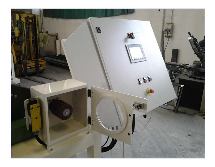
This is an automatic machine for the speed testing of non-woven flap discs and wheels.
