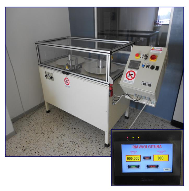
A rewinder and meter counter for rolls.
