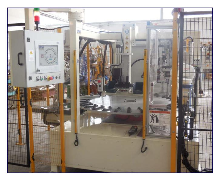
Robotic automated machine for the gluing of shaft mounted flap wheels.
