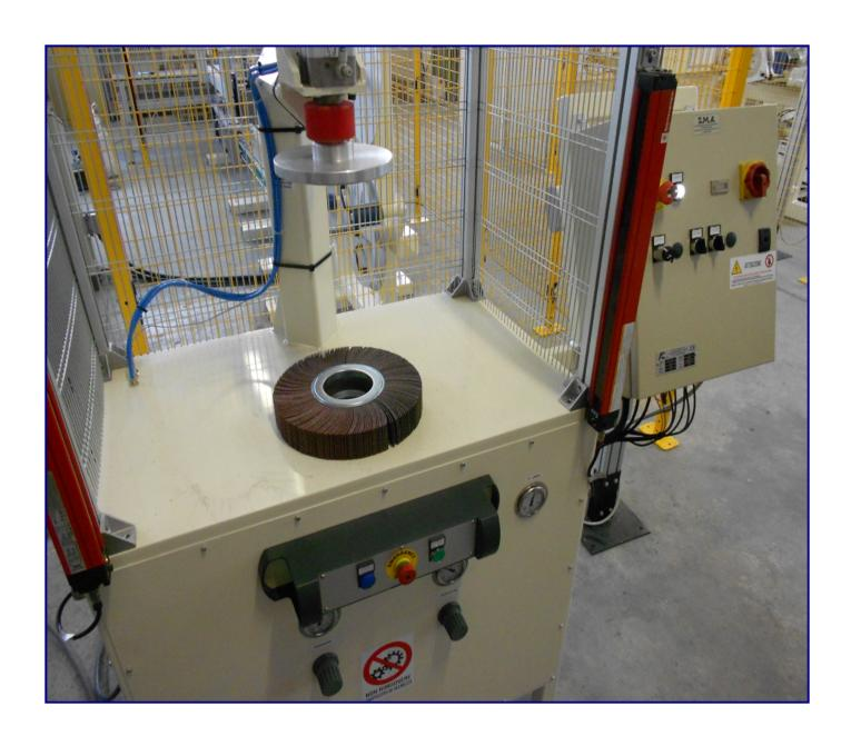
This equipment provides an automatic working process for the pressing of cloth wheels with flange.
