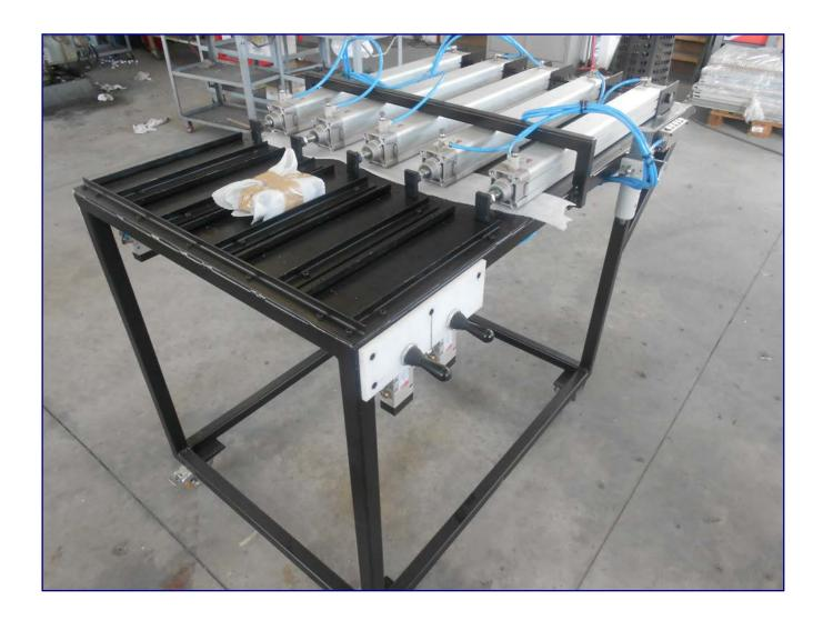
Mobile workbench for the forming of abrasive cloth wheels, in 100x100 and 100x50mm sizes.
