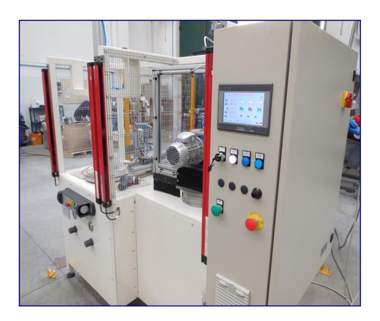
This combo system is designed for the pressing, bonding and centrifuging of wheels. It is controlled by a multifunction PLC with an operator panel that supervises all the working processes. This system is divided into two workstations: one for the bonding and pressing, the other for the centrifuging.
