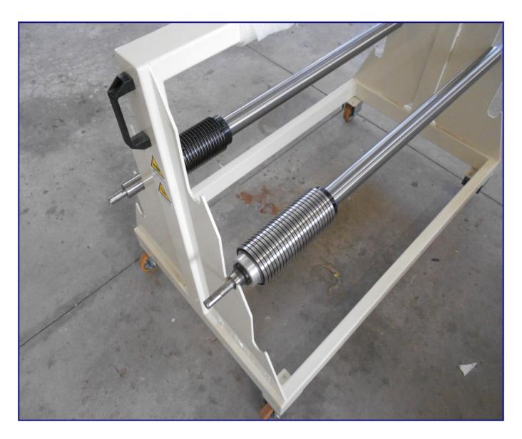
A wheeled, 6-position trolley for shafts.
