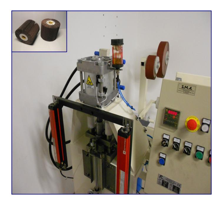
This is a semi-automatic equipment for the production of abrasive cloth wheels whose diameter is  $\emptyset$  100 mm. The abrasive cloth is sheared into flaps, and they are subsequently stored in a vertical loader. This machine is equipped with a panel and a counter that select the number of flaps that have to be cut.
