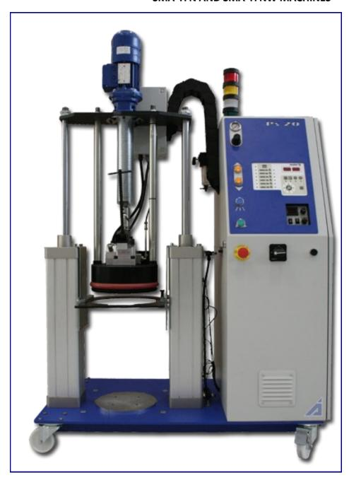
This is a bulk adhesive unloader for PUR Hot-Melt glues.
