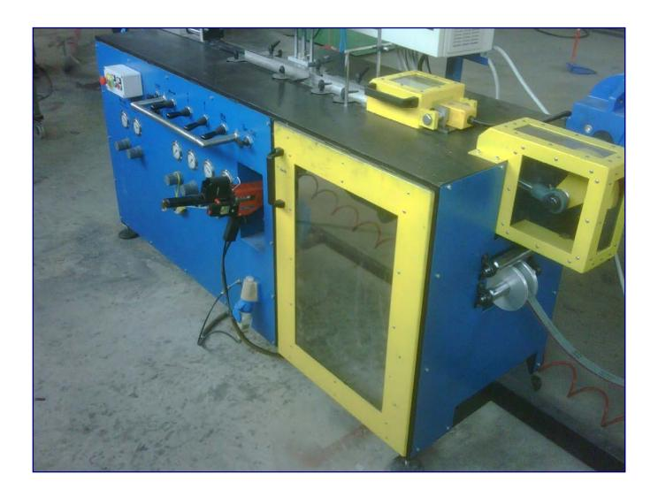
Manual machine for the manufacturing of non-woven wheels whose sizes are 100x100, 110x100, and 120x100 mm; for shaft mounted wheels, diameter goes from 60 to 120 mm.
