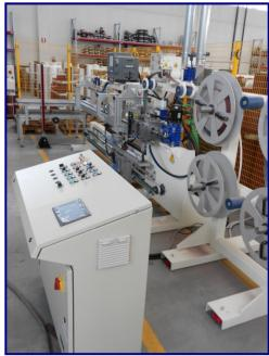
This automatic equipment manufactures abrasive cloth wheels with flange, ranging from 165mm to 350mm diameters, and up to 100mm thickness. This full automatic machine shears and binds abrasive cloth flaps which are subsequently stored in a unit at the end of the process. It is equipped with a multifunction touch screen panel that can set and store all the operator's customised programmes.
