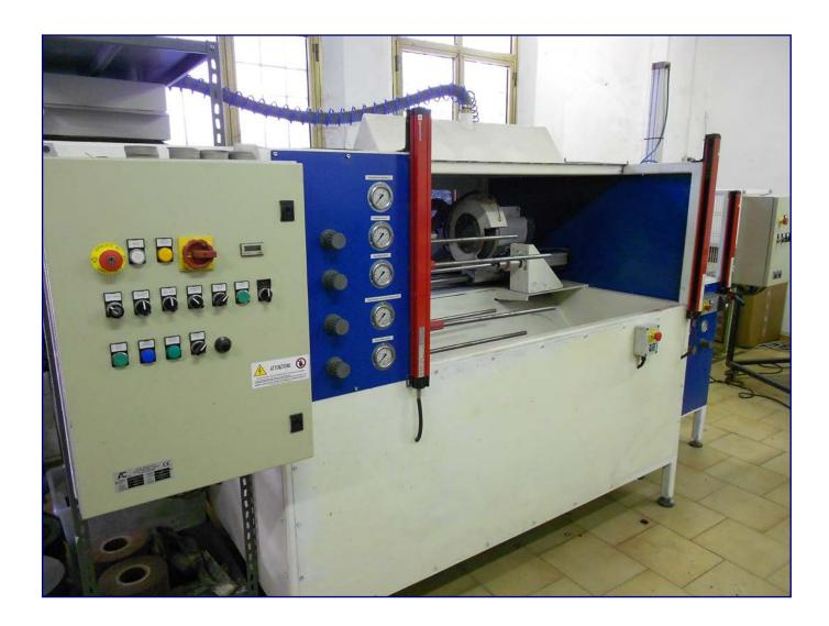
Automatic equipment for the grinding of non-woven wheels.
