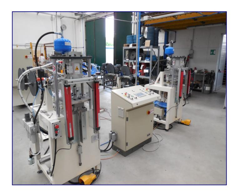
This semi-automatic piece of equipment produces abrasive cloth wheels with flange, ranging from 165mm to 350mm diameters, and up to 100mm thickness. The abrasive cloth is sheared into flaps and they are subsequently stored in a vertical loader. It is equipped with a multifunction touch screen panel that can set and store all the operator's customised programmes.
