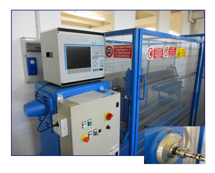
This is a dynamic balancing machine with rigid supports.
