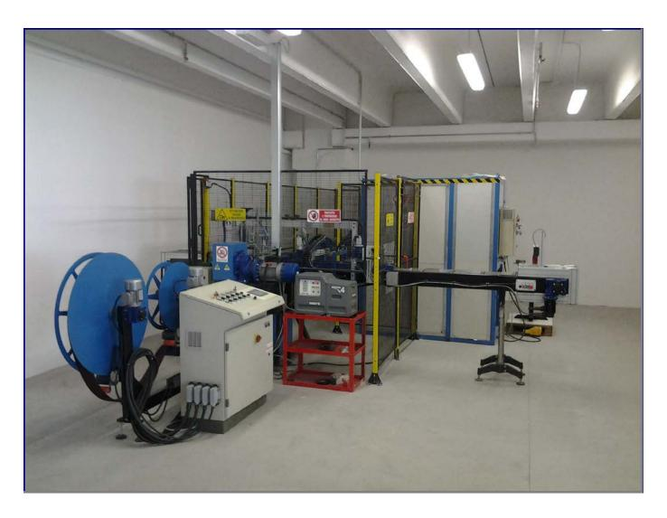
This is an automatic machine for the production of wheels in non-woven fabric and combined non-woven+cloth. Sizes are: diameter 100, 110, 120 mm; height 100 mm.
