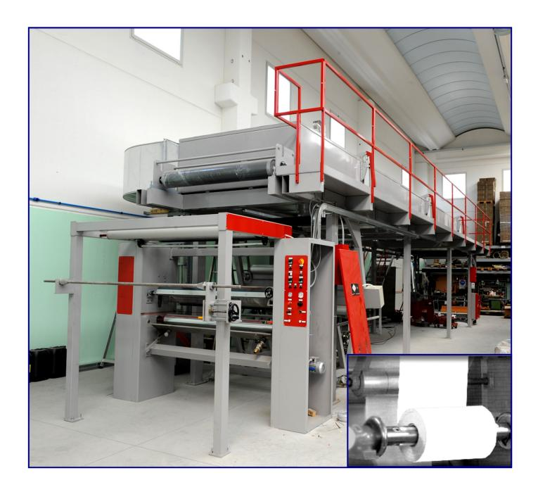
This is an automatic machine for the lamination of abrasive cloth and paper to Velcro® or sponge. This equipment is designed to make large quantities of rolls. Several voltage and alignment sensors automatically control its running, which allows the manufacturing of all kinds of abrasive/non-abrasive cloths and papers.
